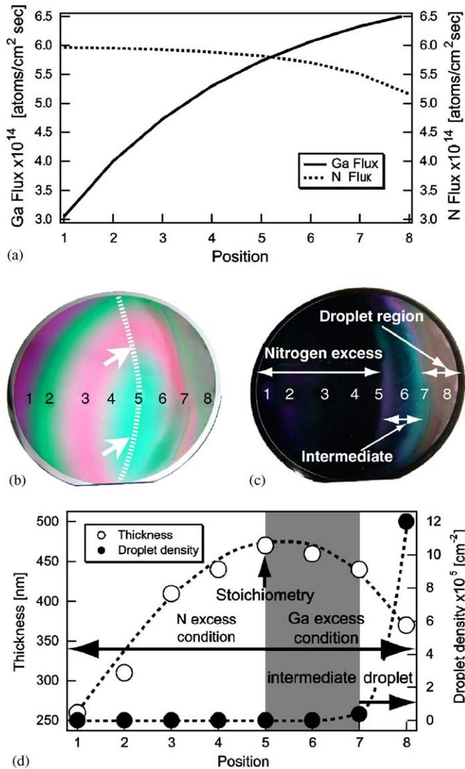
Fig. 3. GaN grown by 'combinatorial growth': (a) distributions of Ga and N flux obtained from Fig. 3(d), (b) interference colors on the sample, (c) illumination of Ga droplet region, (d) distribution of thickness, which were measured from the cross sectional SEM image of the sample, and Ga droplet density.
