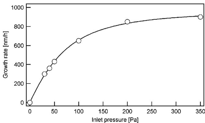
Fig. 5. The inlet pressures dependence of the thickness change of GaN films grown by ‘combinatorial growth’.
