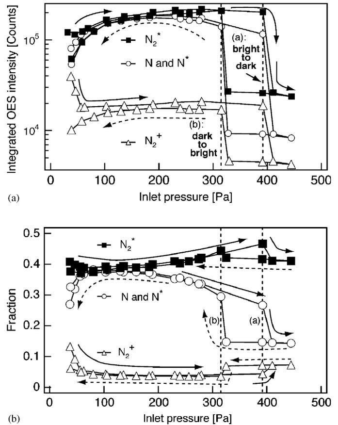
Fig. 4. Relative density and fraction analysis under an RF input power of 400 W: (a) the IOI result, (b) the result of fraction analysis using Eq. (3). Solid arrows show the trend of the increase of inlet pressure and dashed arrows show the trend of the decrease of inlet pressure. The mode shift from bright to dark (indicated as (a)) occurred at 392 Pa whereas that from dark to bright (indicated as (b)) occurred at 315 Pa.
