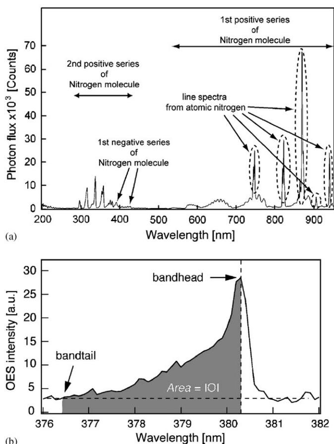
Fig. 2. Nitrogen spectra: (a) results of an OES measurement in ‘bright mode discharge’ typically observed using our RF source, (b) a part of the band spectrum from the 2nd positive series of  $N_2^*$  between 376 and 382 nm. The definition of bandhead and bandtail is shown.
