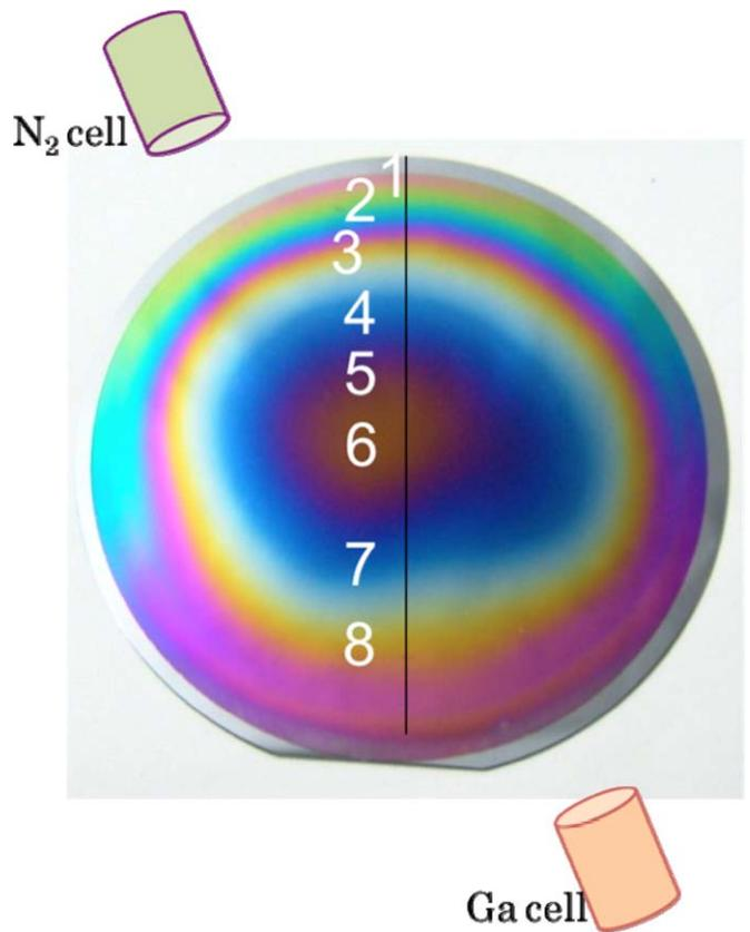
Fig. 7. GaN film grown on 3 inch AlN/Si(111) using AM-MEE under 2 s Ga exposure with 3 s LB (120 W and 70 Pa (1.38 sccm)) discharge and followed by 2 s exposure of the HB (450 W and 70 Pa (1.38 sccm)) discharge without substrate rotation. N and Ga show cells for N and Ga, respectively. The thickness at 1–8 positions are 130, 150, 120, 70, 50, 40, 80, and 150 nm, respectively.
