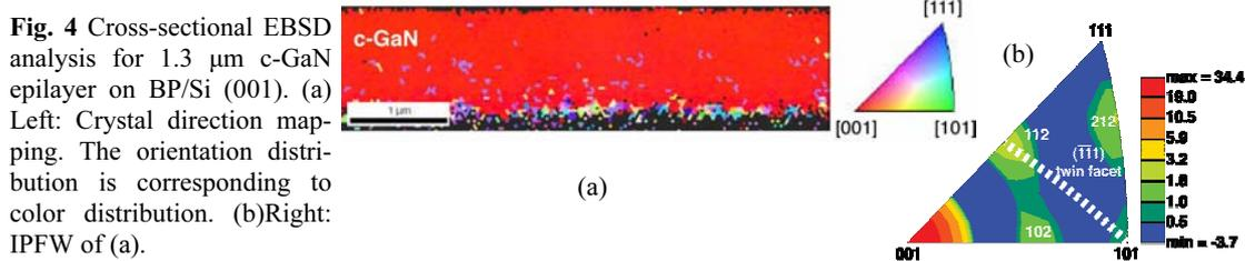
Figure 4a shows the purity analysis results of cross-sectional 1.3  $\mu\text{m}$  thick c-GaN epilayer using x-EBSD method. From the analysis of crystal direction mapping, only 75.6 % of c-GaN was epitaxially grown at the early stage of c-GaN growth including the nucleation layer grown by LT-MEE (0–300 nm). As growth proceeded, the purity of the c-GaN epilayer increased (e.g., the region from 500 to 800 nm thick: 96.7 %, the region from 1000 to 1300 nm thick: 99.4 %).
