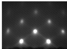
**Fig. 2** RHEED pattern of 10 ML c-GaN using LT-MEE. The azimuth of electron beam was [1-10].
