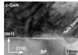
**Fig. 3** HRTEM image of c-GaN. High density of SF and twin feature can be confirmed.
