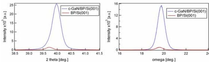
**Fig. 6**  $\theta$ - $2\theta$  (a) and  $\omega$  (b) XRD profiles of c-GaN/BP/Si (001) and BP/Si (001), respectively.  $\omega$  FWHM values: 30.34 arcmin for c-GaN and 28.52 arcmin for BP,  $2\theta$  FWHM values: 14.12 arcmin for c-GaN, and 11.45 arcmin for BP.
