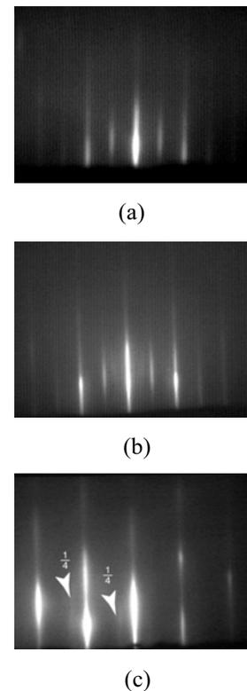
**Fig. 5** RHEED images of c-GaN epilayers. (a) 1.3- $\mu\text{m}$ -thick layer, (b) 2.5- $\mu\text{m}$ -thick layer, (c) 2.5- $\mu\text{m}$ -thick. (a) and (b) were grown under Ga BEP was kept at  $1.03 \times 10^{-4}$  Pa, (c) was grown under  $1.01 \times 10^{-4}$  Pa corresponding to stoichiometric condition.
