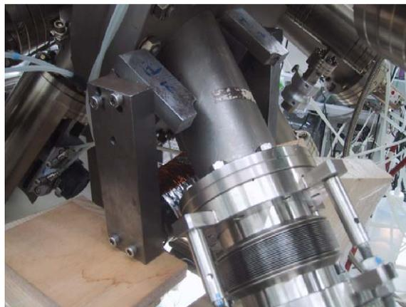
Fig. 1. An electromagnet attached to an RF nitrogen radical port in VG80H MBE chamber.
